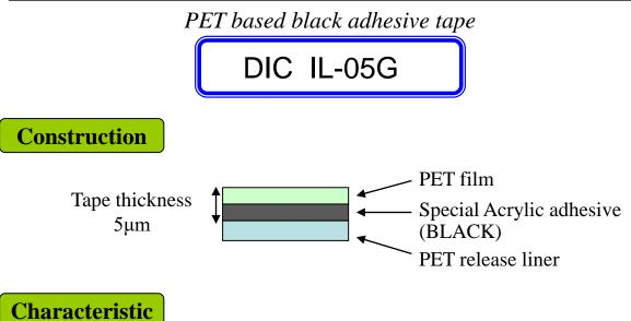
•PET based black adhesive tape. Tape thickness is 5 µm.
