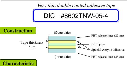
•Very thin! Tape thickness is 5 µm.
