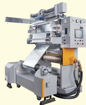
(left) Applications for DUALAM TM include food products and household goods (right) Lamination system
