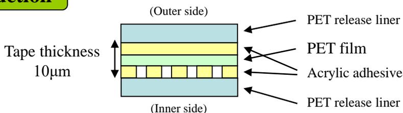
**Remark) Outer side: bonding for graphite sheet. Inner/core side: bonding for adherend.**
