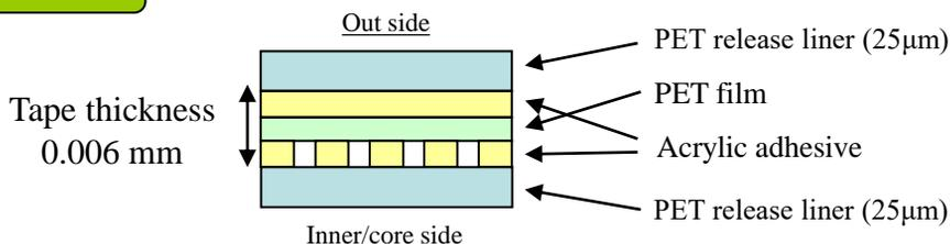
**Remark) Out side: bonding for graphite sheet. Inner/core side: bonding for adherend.**
