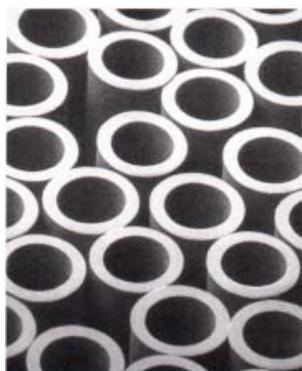
Cross section of a hollow-fiber membrane (magnified)
