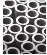
Cross section of a hollow-fiber membrane (magnified)
