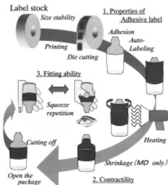
Fig.1 Process of shrinkage adhesive label.
