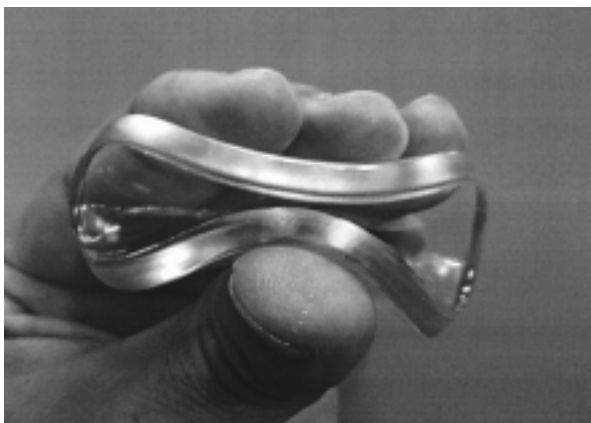
Fig.1 Cured resin of EPICLON EXA-4850-150 on TETA (Tri ethylene tetramine) curing system.
