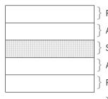
Paper release liner Acrylic adhesive Strong non-woven fabric Acrylic adhesive Paper release liner XOutside of a roll
